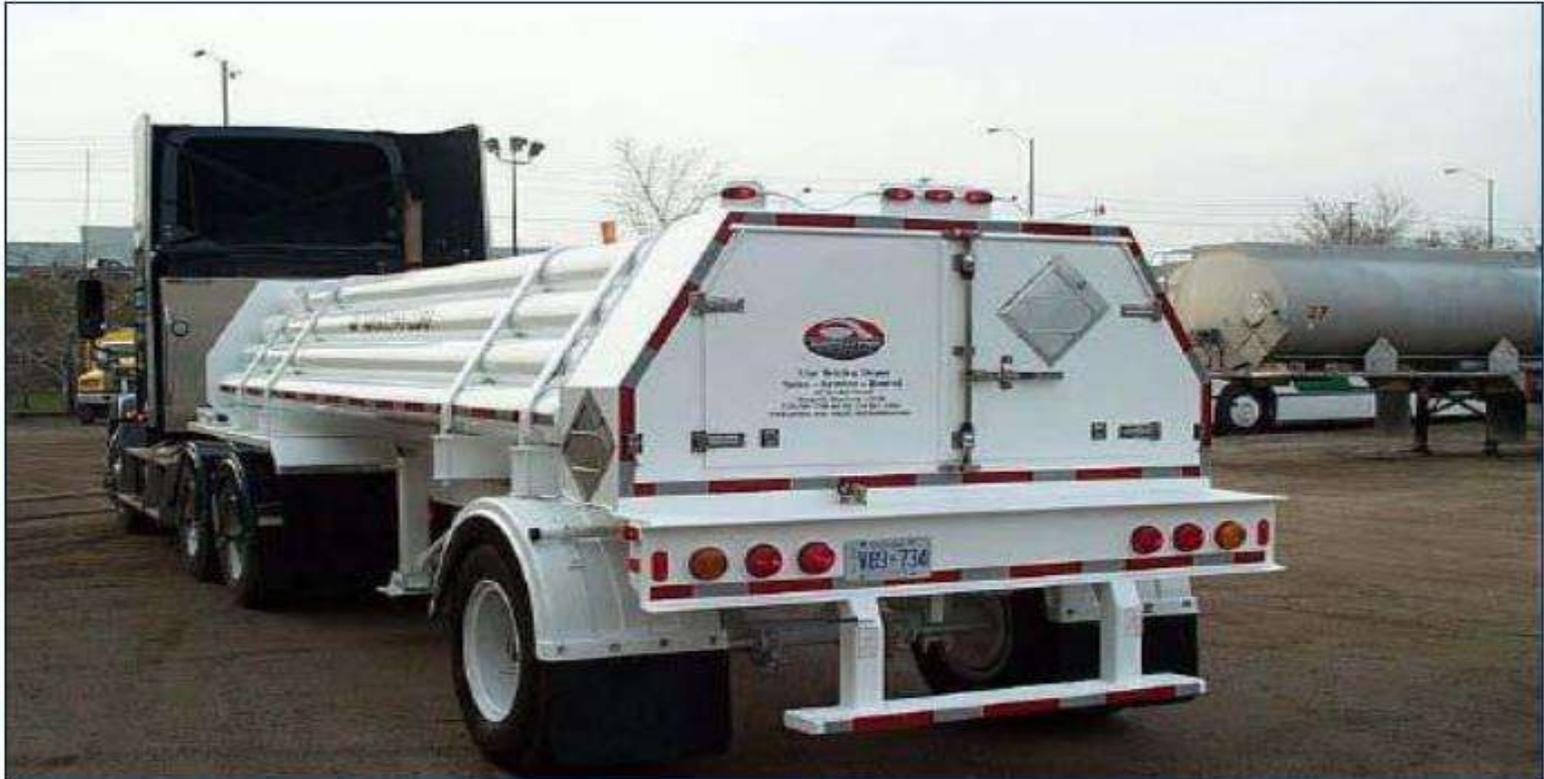
Figure 9: Compressed Hydrogen Gas Tube Trailer – 30 Cylinders and 43,260 SCF (105 kg) Capacity
