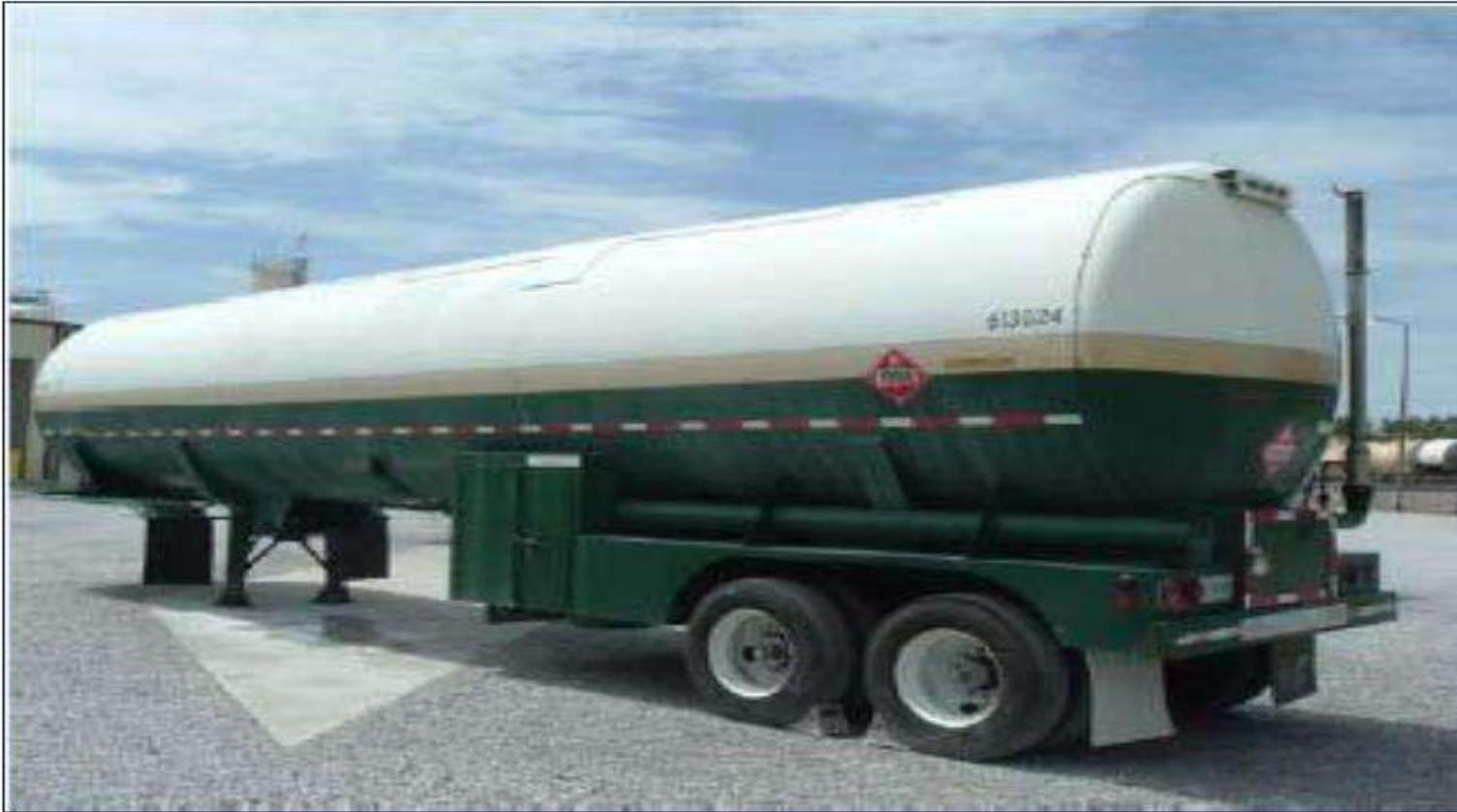
**Figure 10: Cryogenic Liquid Hydrogen Trailer – 13,000 gallon (3,500 kg) capacity**
